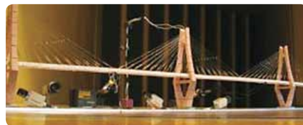
3-D Aeroelastic model test – Cable-Stayed Bridge
