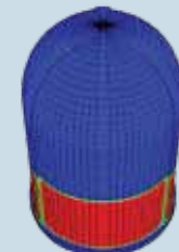
Temperature in a fire-exposed containment building
