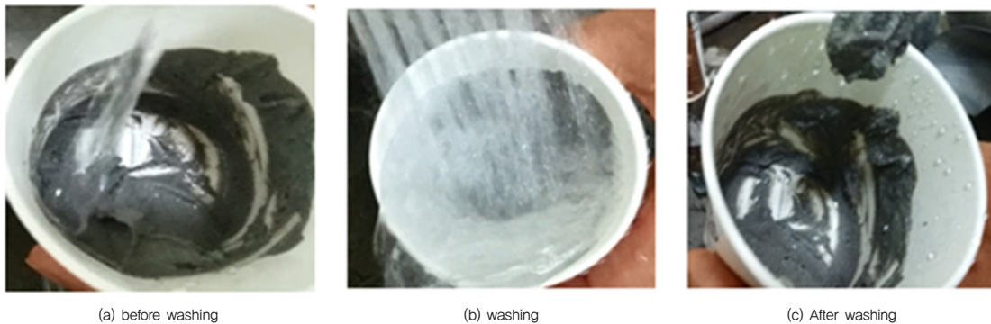
Fig. 2. The anti-washout property of inorganic water-stop agents
