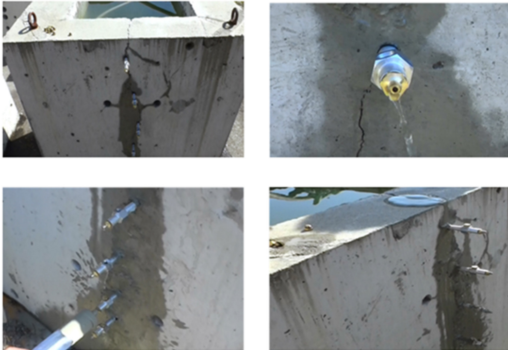
Fig. 9. Effects of water stop by injection of inorganic water-stop agents
