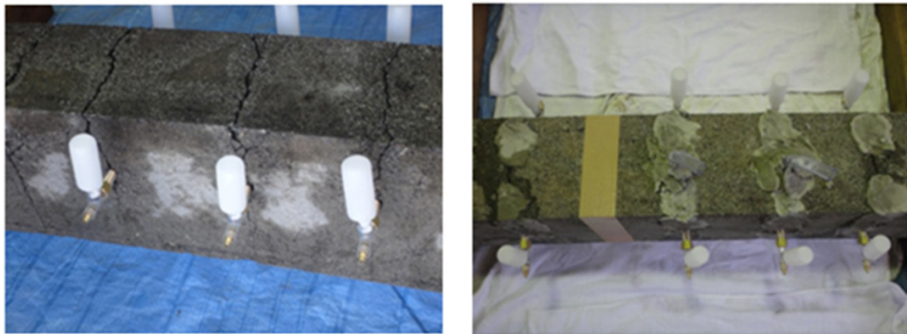
Fig. 7. Surface finishing for the plug installation and injection of inorganic water-stop agent
